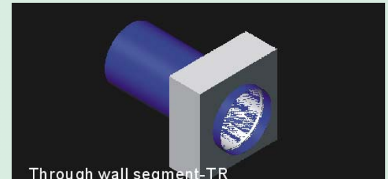
Through wall segment — TW
